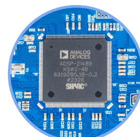
High Performance Fourth Generation Analog devices SHARC Audio Processor
